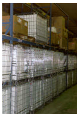
Figure 6.13 Correct: packaging material sealed in plastic and stored in a clean environment.
