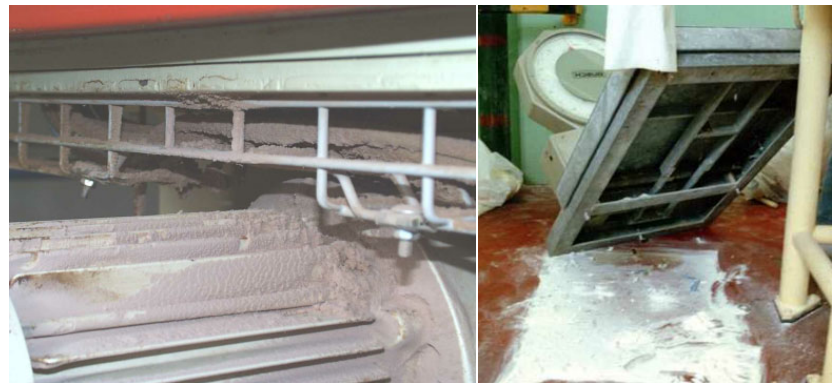
Figure 4.13 Left: underside of process line difficult to clean. Right: effect of balance being attached to the floor.
