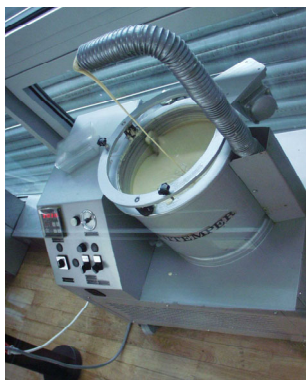
Figure 4.4 Left: Chocolate melting. The lack of a top cover poses a risk of entrance of particles/microorganisms. Right: Lines with open products or packaging should be covered like this to prevent entrance of contaminants in the cans and subsequently in the product
