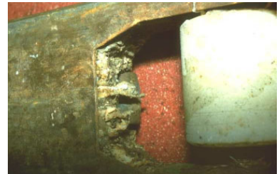
Figure 4.11 Wheels of fork lift may accumulate product residues.
