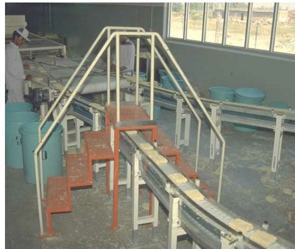
Figure 4.9 Open staircase where people can contaminate the product.
