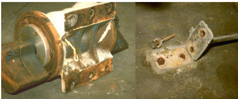
Figure 4.12 Collection of dirt and corrosion under equipment supports.
