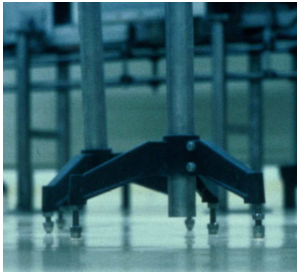
Figure 4.18 Sealing of equipment to floor.
