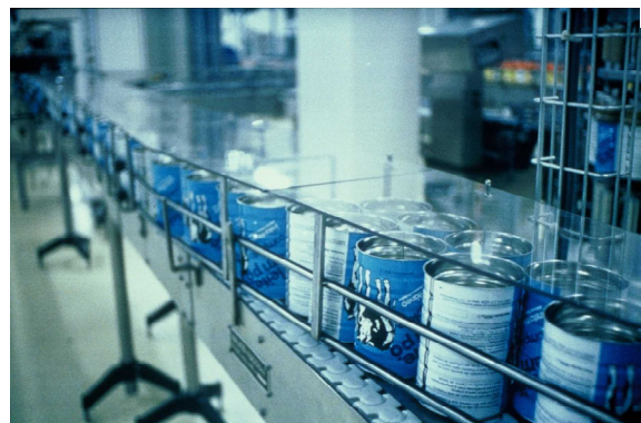
Figure 4.4 Left: Chocolate melting. The lack of a top cover poses a risk of entrance of particles/microorganisms. Right: Lines with open products or packaging should be covered like this to prevent entrance of contaminants in the cans and subsequently in the product
